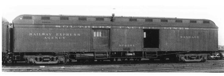
Nine cars built by AC&F in 1906 numbered SP 6284 - 6293, lettered Southern Pacific Lines. The lettering for these cars dates from 1940 with REA as the contract express company. With very slight modifications, this car can be modeled using Ultrascale kit #613.
